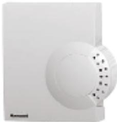
Sensors that measure the CO<sup>2</sup> concentration in the ventilated space or duct. The sensors are used in ventilation and air conditioning systems to control the amount of fresh outdoor air supplied to maintain acceptable levels of CO<sup>2</sup> in the space. Non Dispersion Infrared (NDIR) technology used to measure carbon dioxide gas.
