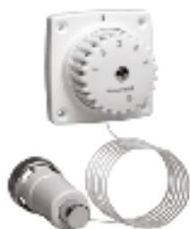
The T100MZ radiator thermostat consists of a thermostatic radiator valve head with a remote liquid-filled sensing element and setting unit. Suitable for all Honeywell thermostatic radiator valve bodies. For use in warm water heating systems.
