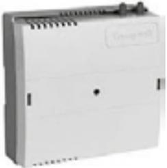
Variable Air Volume (VAV) controller in the Excel 10 family. Using single and dual duct application these VAV systems provide pressure independent or pressure dependent air flow control and series or induction fan control. VAV systems generally provide cool air only to the zones. The W7751 controllers provide additional outputs that control VAV box reheat coils. The heaters can be staged electric or modulating hot water. Supply and exhaust pressurisation control are provided on a zone basis.
