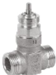
2-way valve for modulating control of hot/cold water in HVAC systems. Specially suited to high pressure and high temperature. Flat/gasket sealing ports. Normally closed and pressure balanced. External threaded BSPP connections.
