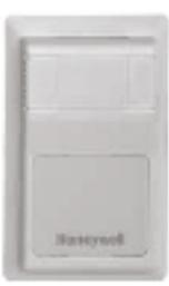
H7625, H7635 are highly accurate and stable humidity transducers designed for use with HVAC controllers such as T7350 thermostat and the T775U Universal Controller. Ceramic technology allows the sensor to recover fully from condensation, fog and high humidity. Temperature compensated output.
