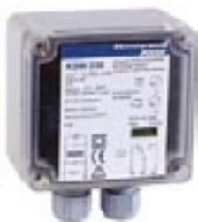
The high reliable compact electronic flow switch is designed for detecting water flow in pipes. As soon as the flow speed exceeds or falls under the adjustable setpoint value, the device will switch an electric circuit.
