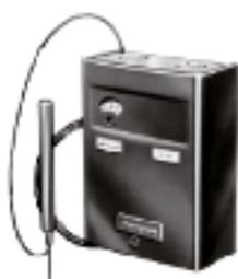
Proportional temperature controllers for modulating control of boilers. Liquid filled copper elements with 1/2in diameter sensing bulbs. 0-135 Ω output. Has end switch to cycle burner on and off at low fire.
