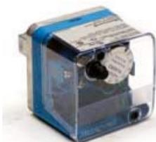
The C6097 pressure switch is used to detect the pressure of gas or air. The switch performs the ON/OFF control of the external electrical circuit in accordance with the set point. This switch can be widely used to detect the upper limit or lower limit pressure of the gas or air to be supplied to a gas combustion system, or detect the clogging of the interlock filter of a burner blower
