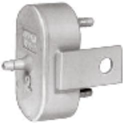
A three port relay used in HVAC systems, averages the signals from two thermostats to control a single device such as a heating coil valve for a multi-zone unit. The pneumatic averaging relay provides an output pressure equal to the average of the two input pressures.
