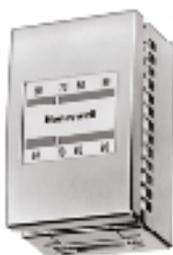
Two-pipe, one or two temp pneumatic thermostat used to provide proportional control of pneumatic valves and damper actuators in heating and air conditioning systems with summer/winter changeover.
