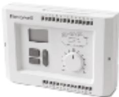
A series of configurable digital controllers for valve or damper control in air or water temperature applications. Functions can consist of main temperature control, limit control, cascade control or outside air compensation control. Floating, PWM or modulating models available. 24Vac.
