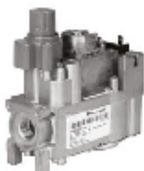
European; Compact combination gas valves, comprise a pilotstat, operator and pressure regulator. Standing pilot application. Low voltage versions(24 Volt) also available. Uses V404 operator and V5306 regulator
