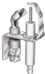
Non-primary aerated, intermittent pilot burner with integral electrode for sparking and flame sensing. For Natural and LP Gas-Fired Equipment.
