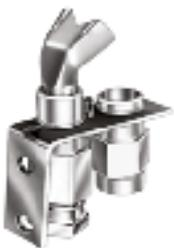
Non-primary aerated insert, orifice-type pilot burner for main burner ignition with Q340 or Q390 thermocouple. Use in Pilotstat safety control operation. For natural and LP gas-fired equipment. Mounting: A-type or B-type. C/W Electrode Clip (for 61023/... Ignitors).
