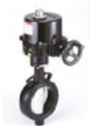
The V4ABFW actuated wafer type butterfly valves are suitable for heating and cooling applications. They can also be employed for industrial applications, general services and water treatment. Cast iron (DN50-150) or ductile iron (DN200-600) wafer body, stainless steel shaft and epoxy coated ductile iron disc. Continuous position indicator.
