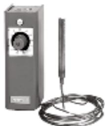
Has 2 SPDT switches that operate in sequence. Adjustable interstage differential and individual switch differential. Switches rated 8.3FLA maximum total per controller. 1/2in diameter sensing bulbs.
