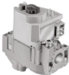
Low capacity (20-200cf/h. 0.56-5.6cm/h) combination gas control, 24Vac 50/60hz regulated main gas (adjustable pilot). Valves for standing pilot, intermittent pilot and direct ignition.
