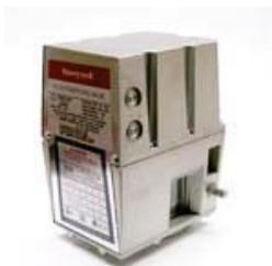
The V4055 gas valve actuator in combination with the V5055 gas valve controls the gas supply to commercial and industrial burners. Use where smooth light off is important, one second maximum closing time, always displays the valve position when open a red indicator appears, when closed yellow indicator appears.
