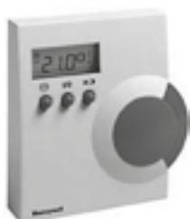
The T7560 Digital Wall Module is a family of direct wired wall modules that display space temperature and provide setpoint, occupied/unoccupied override and fan mode/speed selection for the Honeywell Excel 10 controllers.
