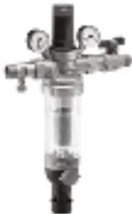
HS10S combination water supply units integrate a non-return valve with test point, reverse rinsing fine filter, pressure reducing valve and shut-off valve in one appliance. They ensure a continuous supply of filtered water.
