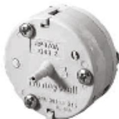
Direct acting, modulating relay provides increased capacity of the branch-line pressure to the final control device. Max operating pressure: 205 kPa (30psi).
