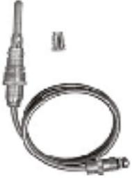
Universal thermocouple individual blister pack. 60 sec drop out. C/Q Clip and Adapter. Made in USA and suits mainly American pilot brackets. Average operating life of ten years. Available in variety of lead lengths (18" to 48"; 0.5m to 1.2m).
