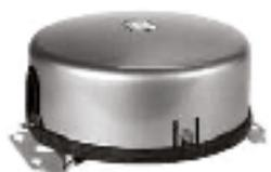
One-pipe, direct or reverse acting pressure sensor used with RP920 controllers to provide control of duct static, velocity or differential pressure in airflow applications. Duct mounting.
