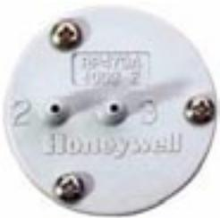
Three port relay used in HVAC systems to perform a variety of relay functions; transmit the higher of two input signals, lock out one pressure signal when second signal is higher, or transmit the lower of two pressure signals.
