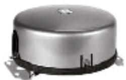
One or two-pipe, direct or reverse acting, low or high capacity controller used with pneumatic actuators to regulate static or differential pressure in central fan installations. Adjustable setpoint and throttling range.
