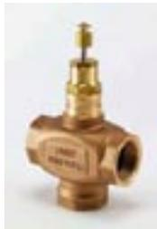
2-way single seated control or shut-off valve with yellow brass body and stainless plunger. Application for hot water, chilled water, domestic hot water, saturated steam, superheated steam in HVAC. Internal threaded BSPT connections.
