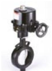
The V4BFW actuated wafer type butterfly valves are suitable for heating and cooling applications. They can also be employed for industrial applications, general services and water treatment. Cast iron (DN50-150) or ductile iron (DN200-600) wafer body, stainless steel shaft and epoxy coated ductile iron disc. Continuous position indicator.
