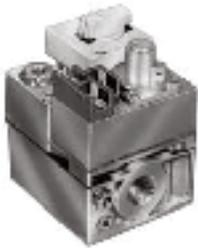
Single block combination gas valves for standing pilot applications. Use V804 operators and V530xx regulators. 24Vac. Eco's available (Part No: 392490-2).
