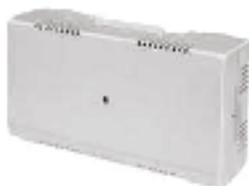
The Excel 15A W7760A Building Manager is a LonMark compliant device that can be used to monitor and control HVAC equipment and other miscellaneous loads in a distributed network. An optional lithium battery can be installed to allow continuous power so trend logs and alarms can be maintained for up to 4 continuous years. The W7760A Building Manager communicates via the 78kbaud Echelon LonWorks Network using a free topology transceiver (FTT).
