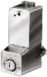
Two-pipe, single temperature, pneumatic temperature controller provides proportional control of pneumatic valves and damper actuators in heating and air-conditioning systems. Adjustable setpoint and throttling ranges.
