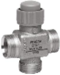
3-way small linear valve for individual room control, small reheaters, coolers and fan coil units. Normally closed. Conical sealing end connections. External threaded BSPP connections.
