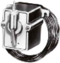
One-pipe, direct-acting temperature sensor used with RP920 controllers to provide proportional control of pneumatic valve or damper actuators. Averaging, liquid filled element for duct mounting. Easily formed into variety of configurations to assure sensing of average temperatures.
