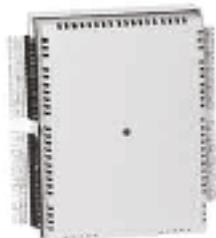
The Excel 15C W7760C Plant Controller is used to monitor and control HVAC equipment and other miscellaneous loads in a distributed network. The W7760C Plant Controller communicates via the 78kbaud LonWorks network using a free topology transceiver (FTT). LonSpec software is used for easy programming.
