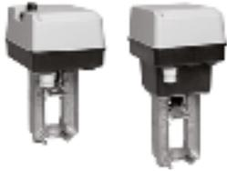
Electric Actuators for floating or modulating control of valves in heating and air conditioning systems. 24Vac 50/60 Hz. Compatible valves; V5011; V5013; V5049; V5050; V5328; V5329; V5088.
