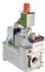
European, compact, automatic combination gas control which performs all the functions required to safely regulate gas flow to the pilot burner and the main burner of; domestic central heating equipment, warm air furnaces, back boilers and water heaters. Redundant intermittent pilot, direct ignition valves and various regulator options available. 24Vac operation.
