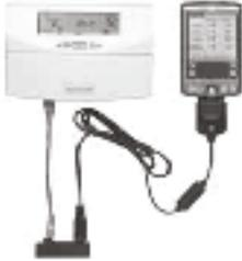
7 day programmable electronic thermostat, with 4 periods/day. Features Intelligent Fan; Intelligent Recovery. Used for heat pump or conventional applications with auto or manual changeover option. Integral or remote sensor. Optional discharge sensor and outdoor sensor. Optional motion sensor. 24 Vac.
