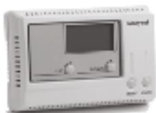
Smartronic is the ideal controller for 2 or 4 pipe fan coil units or heat exchangers. Used with a NTC20K sensor, it controls modulating and/or switched outputs. 24Vac.
