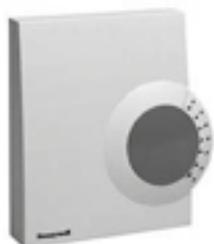
Direct wired wall module for use with the Honeywell Excel 10 devices. All models have a space temperature sensor, some models have setpoint adjustment, bypass button and LED and fan switch. 24Vac 50/60Hz.
