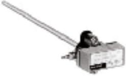
One-pipe, direct-acting temperature sensor used with RP920 controllers to provide proportional control of pneumatic valve or damper actuators. Rod and tube insertion element for duct, well or through the wall mounting. Corrosion resistant.
