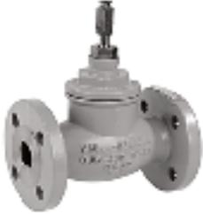
Single seated 2-way flanged valve used for modulating control of chilled/hot water & steam. Nodular iron body, Stainless plug, stem and seat. Noise optimised and balanced, these valves are specifically designed for high differential pressure applications. Replaces V176A valves.
