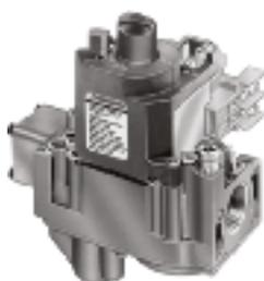
Medium capacity(30-300cf/h. 0.85-8.5cm/h) Combination Gas Control. 24V 50/60hz regulated main gas (adjustable pilot) valves for standing pilot, intermittent pilot and direct ignition.
