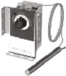
Two-pipe, single temperature, unit mounted, remote bulb pneumatic thermostat used to provide proportional control of pneumatic valve and damper actuators in heating and air conditioning systems. Liquid filled remote bulb.
