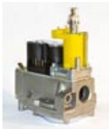
Gas control for combined valve and ignition system(CVI), developed for gas fired appliances with either intermittent pilot or direct burner ignition. Designed to work directly with S4565/75/85 series ignition controllers. Combined system provides programmed safe light up, flame supervision and gas flow regulation. Note that ignition modules are ordered seperately.
