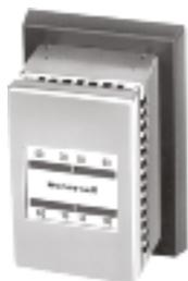
Two-pipe, single setpoint, pneumatic thermostat used to provide proportional control of pneumatic valves and damper actuators in heating & air conditioning systems.
