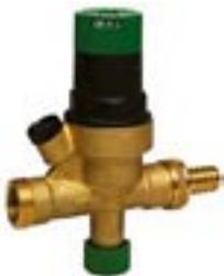
The VF06 filling valve permits simple and safe filling or refilling of a closed heating system. The VF06 consists of a pressure reducing valve, a check valve and a shutoff facility combined into the one unit.
