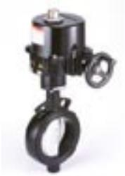
The V4BFW actuated wafer type butterfly valves are suitable for heating and cooling applications. They can also be employed for industrial applications, general services and water treatment. Cast iron (DN50-150) or ductile iron (DN200-600) wafer body, stainless steel shaft and epoxy coated ductile iron disc. Continuous position indicator.
