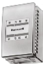
One or two-pipe, single temperature, low capacity, pneumatic thermostat used to provide proportional control of pneumatic valves and damper actuators in heating and air conditioning systems. For 1 pipe functionality, order external 0.0005in restriction 14002913-001.
