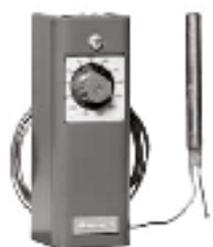
Provide limit or temperature control in refrigerated areas where remote mounting of the sensing element is required. Liquid filled copper elements with 3/8" diameter sensing bulbs.
