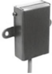
The H7018 early warning dew-point sensor is designed for use in monitoring cooling water pipes or chilled surfaces in order to determine if temperatures are approaching the dew-point. The sensor measures the relative humidity prevailing directing at the chilled surface. Can be used with W7763C chilled ceiling controller.
