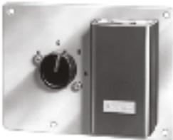
Enthalpy control that senses total heat (humidity & temperature) of outside air. Features nylon humidity sensor. Liquid filled temperature sensing bulb. With mounting plate and adjustment knob.
