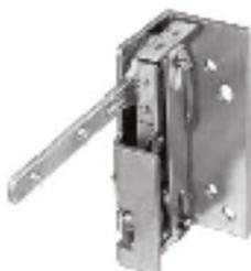
One-pipe, single temp, low capacity pneumatic thermostat used to provide proportional control of pneumatic valves and mixing boxes in heating and air conditioning systems. Mounts in a slot/ light troffer diffuser or a return air grill. Two-way setpoint indicator for vertical or horizontal mounting.
