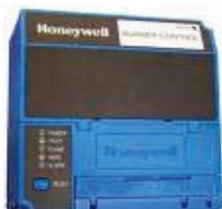
Microprocessor-based integrated flame switch for detecting a flame using rectification, ultraviolet (UV) or infrared (IR) source. Provides level of safety, functional capability and features beyond conventional controls. Use with flame signal amplifiers R7847, R7848, R7849, R7851, R7861 or R7886
