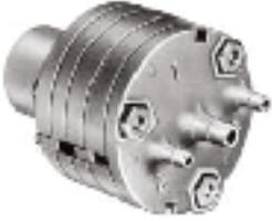
A modulating relay suitable for all types of heating and air-conditioning control systems to reverse and increase the capacity of the branchline pressure to the final control element. The output varies inversely with the input, with an adjustable offset.
