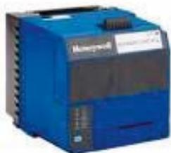
The EC/RM7800 Series is a microprocessor based burner programmer suitable for all types of flame detection systems. The burner programmer is of modular design and can be upgraded with various communication options. All relay modules require a sub base, flame amplifier and purge card. EC=230Vac. RM=120Vac.
