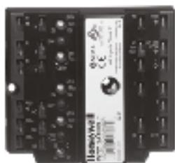
Economiser Logic Module used to adjust the outdoor and return air dampers for control of free cooling in HVAC equipment. Operates from thermostat and CO2 sensor to provide a totally integrated control system. Can be used with TB7220 & TB8220 thermostats, C7632 CO2 sensors and with any Honeywell spring return modulating damper actuator.
