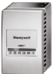
Two-pipe, single setpoint, pneumatic humidistats used to provide proportional control of pneumatic valves on humidification or dehumidification systems. Backplate has molded air connections; no separate fittings needed.
